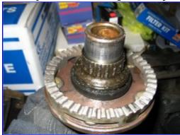
And what it should look like after the inner bearing race and seal are removed:
